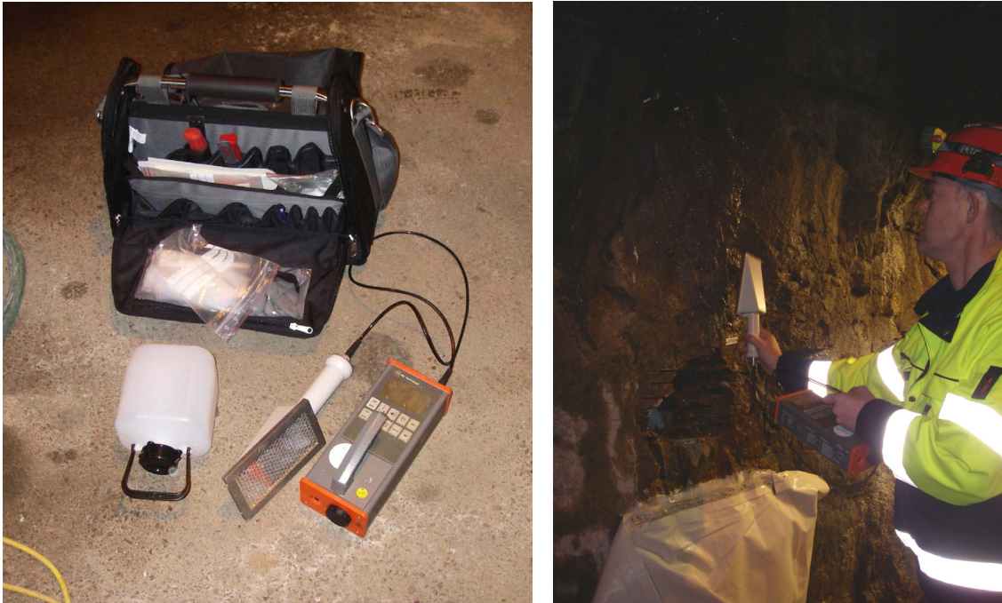
Figure 2-9. a) Equipment used for measurements of radio activity. b) The tunnel wall of TASI is tested by Bjarne Karlsson from CLAB using a scintillation detector (photos: Oskar Sigurdsson).
