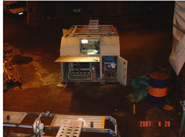
Figure 3-2. a) The BIPS probe and the instrument & control box. b) The instrument & control box. The BIPS probe is inserted in a borehole and connected to the box with a cable (photos: Ch. Gustafsson).
