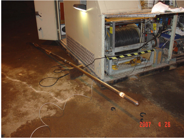
Figure 3-2. a) The BIPS probe and the instrument & control box. b) The instrument & control box. The BIPS probe is inserted in a borehole and connected to the box with a cable (photos: Ch. Gustafsson).
