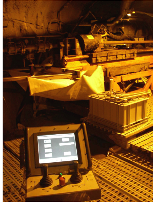
Figure 2-2 a&b. The Onram 2000 CCD computer controlled drill rig used for the core drilling of KI0010B01 (photos: Elinor Örtendahl). a) the rig in position. b) the computer aided control unit.
