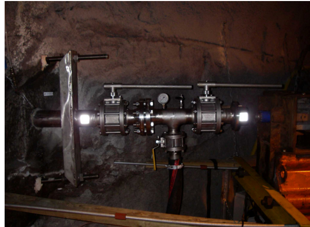
Figure 2-6. The arrangement of the casing and the core drill rig. a) The drill rig is fastened to the tunnel wall by bolts and the drill pipe is in place in the casing (photo: Elinor Örtendahl). b) A close-up of the valve taps and the water pressure gauge (photo: Oskar Sigurdsson).
