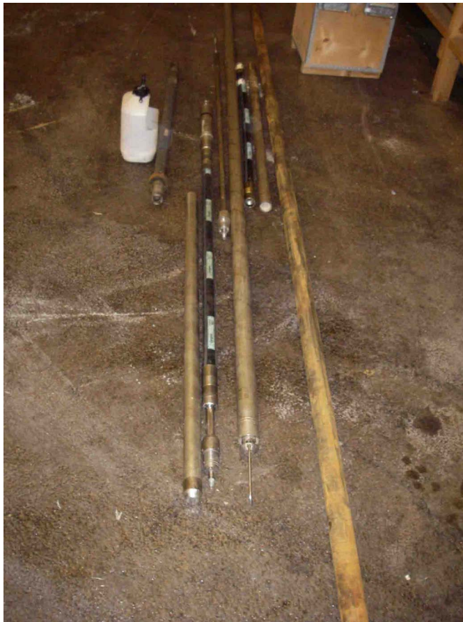
Figure 4-4. a) Double packer to be used at the double packer tests. The packers are not assembled yet (photo: Oskar Sigurdsson). b) Principle sketch of the assembled double packer system, the test unit [modified from Hydrauliskt Testsystem för Underjordsmiljö (“Hydraulic Test system in an underground environment”) Mansueto Morosini 1998, NR TD-98-04, internal SKB document].
