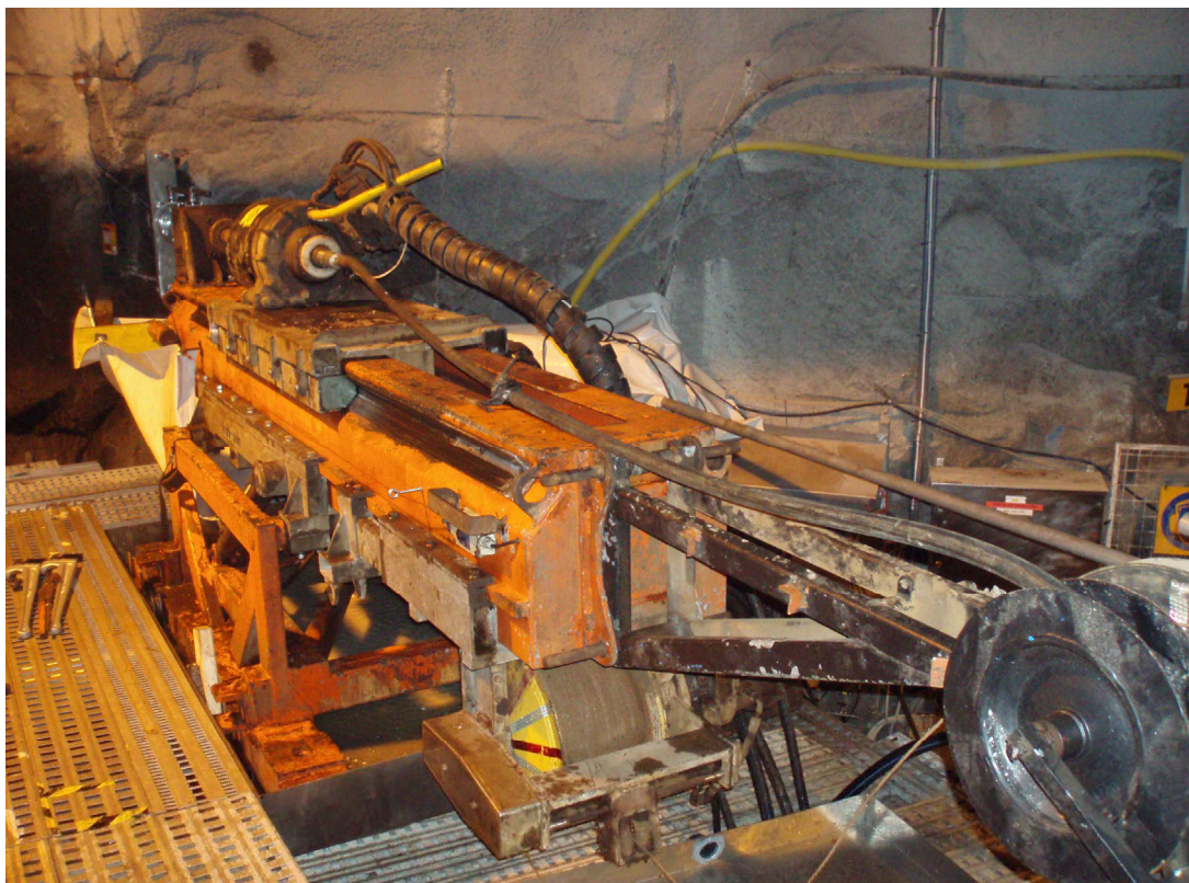
Figure 2-2 c. The Onram 2000 CCD computer controlled drill rig used for the core drilling of KI0010B01. The rig is in position for drilling KI0010B01 (photo: Elinor Örtendahl).
