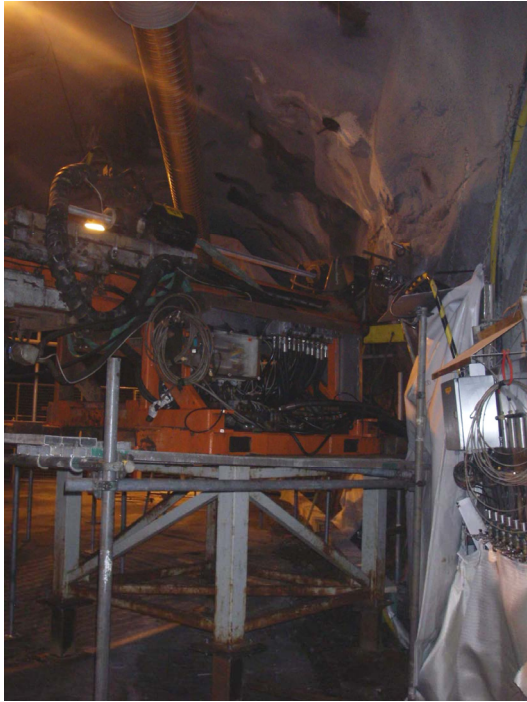
Figure 2-2 a&b. The Onram 2000 CCD computer controlled drill rig used for the core drilling of KI0010B01 (photos: Elinor Örtendahl). a) the rig in position. b) the computer aided control unit.
