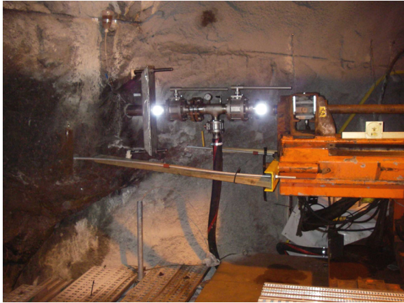
Figure 2-6. The arrangement of the casing and the core drill rig. a) The drill rig is fastened to the tunnel wall by bolts and the drill pipe is in place in the casing (photo: Elinor Örtendahl). b) A close-up of the valve taps and the water pressure gauge (photo: Oskar Sigurdsson).
