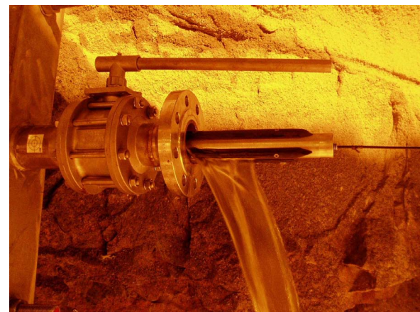
Figure 4-8. a) A close up of the rubber discs on the measuring device. b) The measuring device is almost fully inserted into the borehole via the casing valve and only the guides at the end are visible (photos: Elinor Örtendahl).
