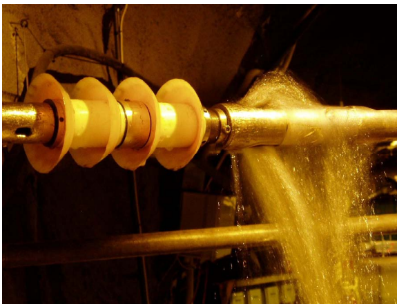
Figure 4-8. a) A close up of the rubber discs on the measuring device. b) The measuring device is almost fully inserted into the borehole via the casing valve and only the guides at the end are visible (photos: Elinor Örtendahl).
